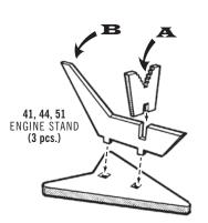
Cement engine stand together as shown above. Display your "extra" engine by cementing its oil pan to point A and transmission to point B.
