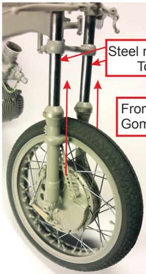
Steel rod  $\varnothing$  3mm x 38mm
