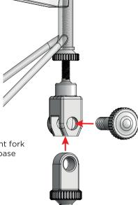
Complete assembling the front fork attachment by installing the base using the fixing screw.
