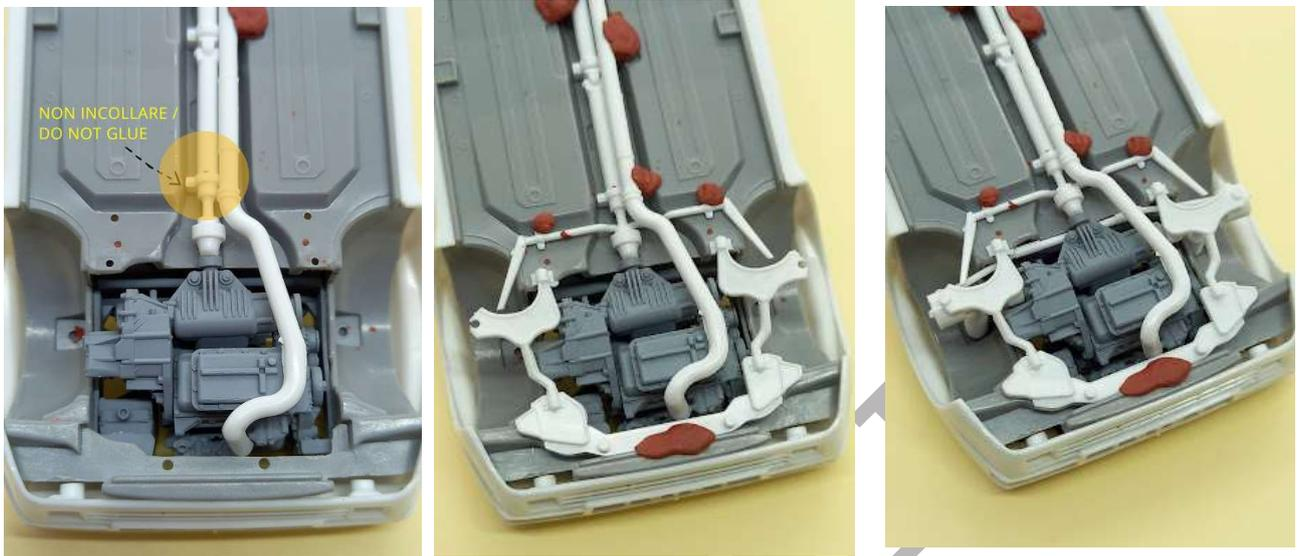
Before fixing the shock absorbers we insert the drive shafts, Also in this case I recommend vinyl glue to be able to find the right angle.
