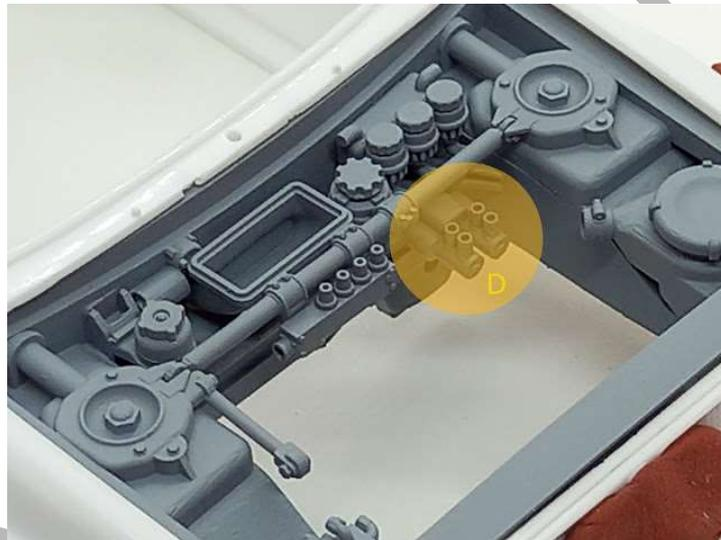
At this point the reinforcement bar of the domes "E" can be inserted (the joints in the two end areas of the bar must be thinned with sandpaper as they are slightly thicker for printing purposes). Also in this case it is advisable first to fix the cables on the control unit which will then be fixed to the spark plugs on the engine head.
