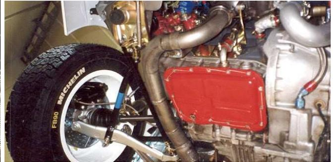
The next step is to install the gearbox with its differential. The starter motor must be fixed AFTER installing the gearbox itself. First of all, it is advisable to go over the housing of the drive shafts with a drill bit as a little liquid resin could remain inside it, which then solidifying could create an obstacle. The drive shafts are recovered from the kit by eliminating the central part (just leave 1/2 mm as in the photo).
