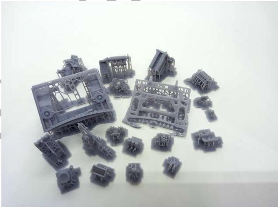
To easily separate the pieces from the print supports, it is necessary to use flat modeling cutters and proceed without haste, cutting one support at a time. When separating the finer parts from the supports (such as the inside of the hood for example) it is necessary to use great caution and press the surface on the opposite side with a finger to avoid breakage:
