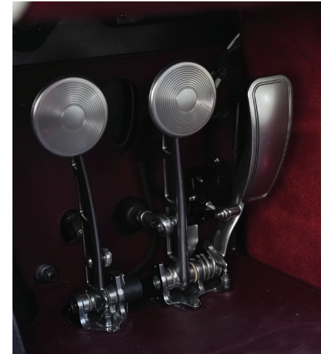
THE FINELY DETAILED PEDALS ARE MILLED FROM A SINGLE BLOCK OF METAL.
