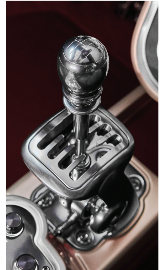
PAGANI UTOPIA USES THE XTRAC 7-SPEED TRANSVERSAL AMT(AUTOMATED MANUAL TRANSMISSION) OR PURE MANUAL, WITH ELECTRO-MECHANICAL DIFFERENTIAL.
