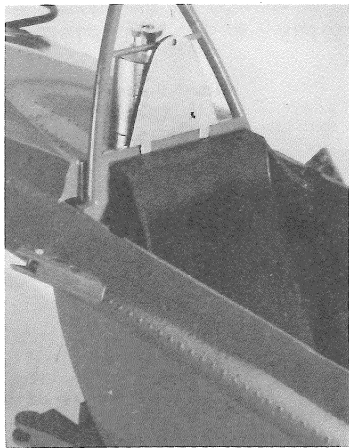
Figure 20. Bulkhead Construction. Fix C2 and the parts which have been assembled in Figure 18 on to the body, and assemble further as shown in the diagram. Allow the coil springs M5 to project out, in the position shown in Figure 21.
