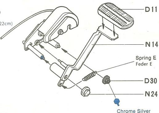
**12** Fixing of Brake Pedal
