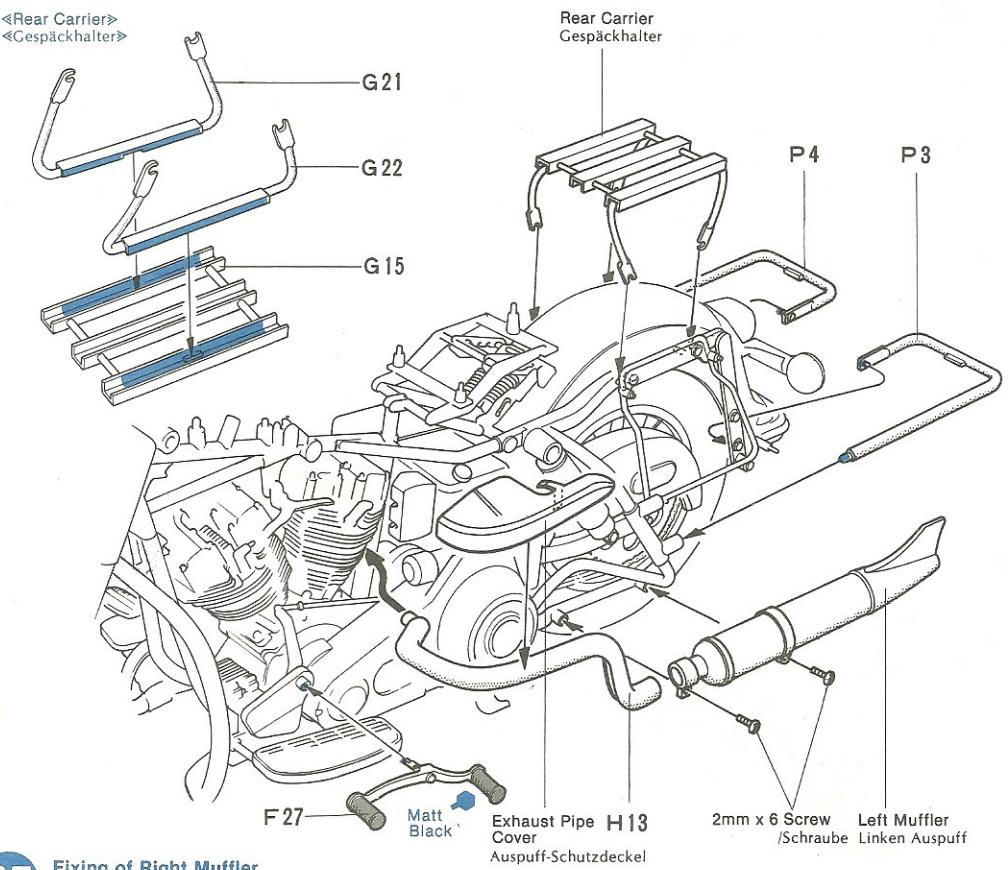
**35** Fixing of Right Muffler
