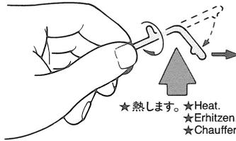
★Heat sprue as shown. Remove from heat and stretch. Allow to cool and cut to required length.
