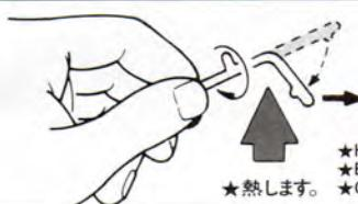
★Heat sprue as shown. Remove from heat and stretch. Allow to cool and cut to required length.
