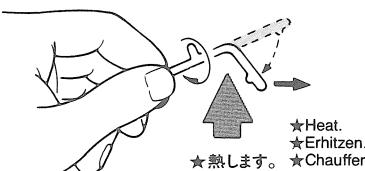
★Heat sprue as shown. Remove from heat and stretch. Allow to cool and cut to required length.
