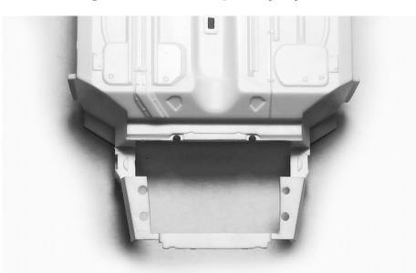
Drill <u>1mm</u> holes in side walls of engine bay:
